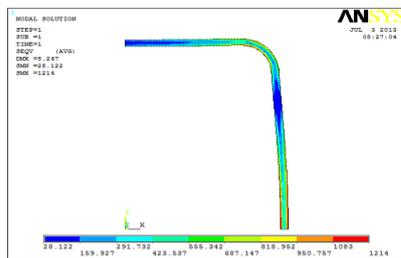
Fig.8: Von-mises stress contour of box 2.5 mm thickness & 10 mm fillet radius
