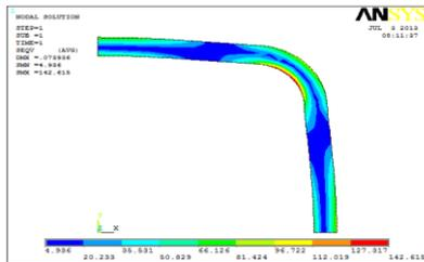
Fig.4: Von-mises stress contour of box 5 mm thickness & 10 mm fillet radius
