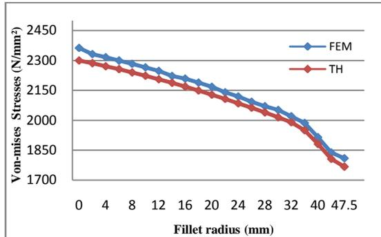
Fig.15: Comparative graphical results for FEM & ANALYTICAL at location A
