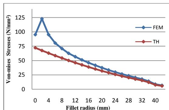
Fig.7: Comparative graphical results for FEM & ANALYTICAL at corner
