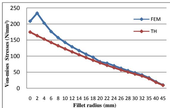
Fig.5: Comparative graphical results for FEM & ANALYTICAL at corner
