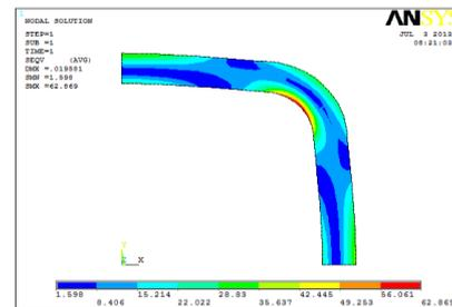
Fig.6: Von-mises stress contour of box 7.5 mm thickness & 10 mm fillet radius
