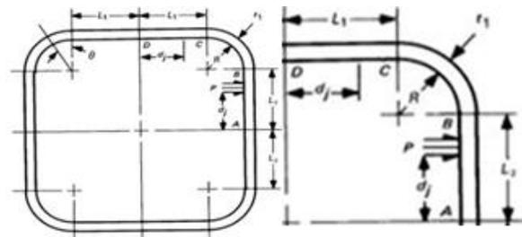
Fig.1: Cross section of rectangular box having uniform thickness & varying fillet radius
