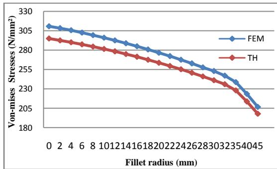
Fig.11: Comparative graphical results for FEM & ANALYTICAL at location A
