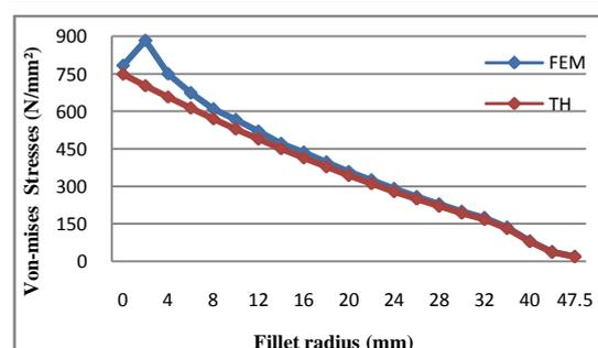
Fig.3: Comparative graphical results for FEM & ANALYTICAL at corner
