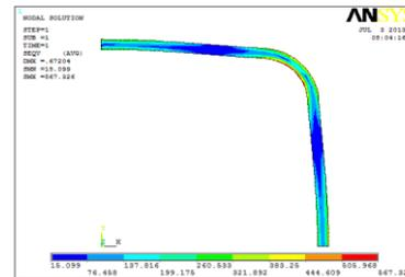
Fig.2: Von-mises stress contour of box 2.5 mm thickness & 10 mm fillet radius
